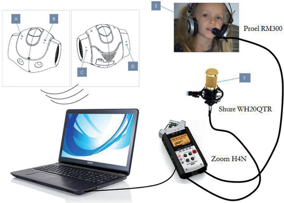
Figure 1 - Data Collection framework: A,B,C,D - 4 microphones of Nao (the robot used in the ALIZ-E project); E - 1 close-talk microphone; F - 1 panoramic microphone
